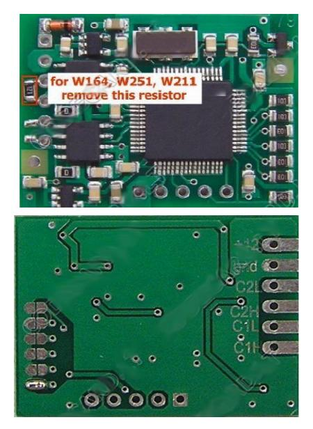
Remove from EZS board SMD part marked with red "X". With short, good isolated wire connect Mercedes CAN filter to EZS board according picture: 1-1 (C1H), 2-2(C1L), 3-3(C2H), 4-4(C2L), 5-5(GND), and 6-6 (+5V).
