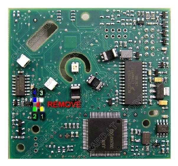
After connection insulate Mercedes CAN filter board with heat shrink or insulation tape. Put it carefully to EZS casing.
